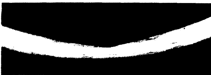
(b) Fig. 6. (a) Measured moment-curvature response (pure bending case). (b) Localized collapse mode.
