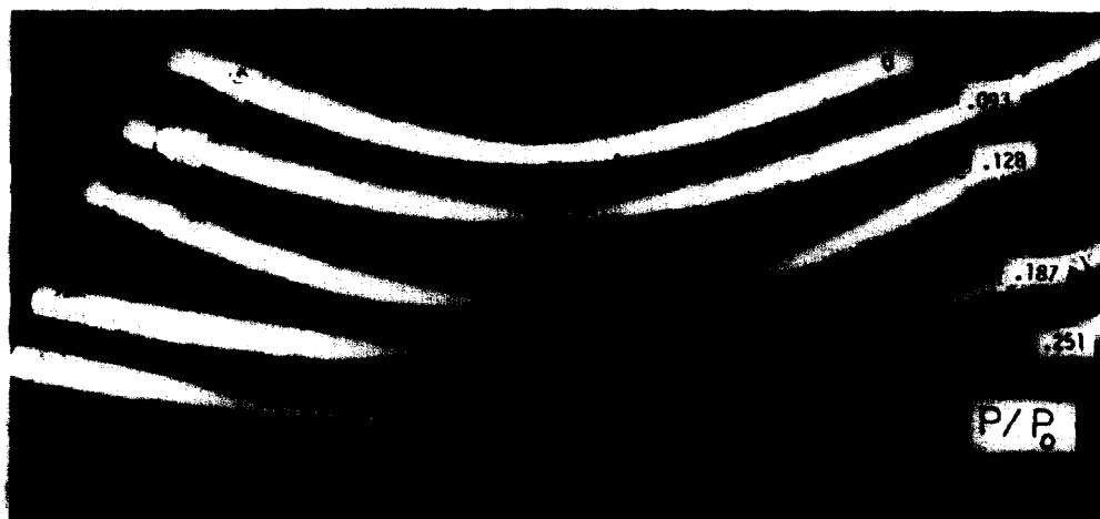
Fig. 9. (a) Measured moment-curvature responses for different values of pressure. (b) Test specimens collapsed at different pressures (and curvatures).
